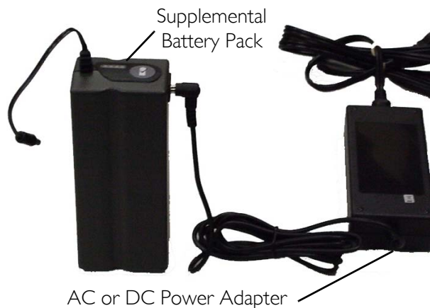
FIGURE 2 Charging the Supplemental Battery
