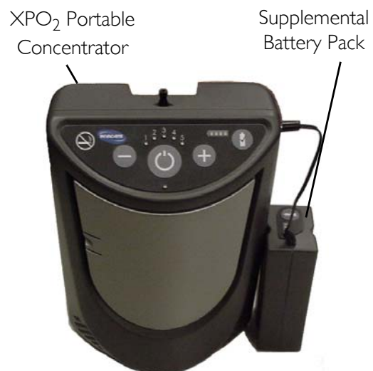
FIGURE 1 Connecting the Supplemental Battery to the XPO 2
