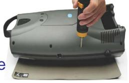
Remove ten #1 Phillips screws from cover & <u>carefully</u> turn unit onto it's back.
