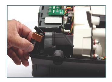
9v battery and adhesive foam tape provided in PM Kit P/N:5022)
